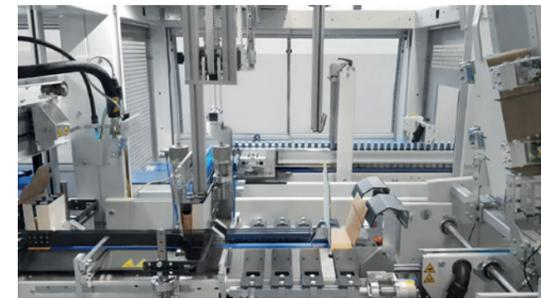
ring a **colour touch screen interface** and management of different components via **gear motors and servomotors**, they provide a high degree of automation and precision that facilitates the management of the entire process. These features enhance **safety and efficiency in the packaging line**, while also reducing the likelihood of errors that could lead to waste, a critical factor in conscious and sustainable production.
