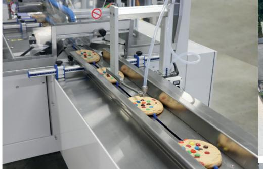
With its high-speed models, it can package up to 200 products per minute.
